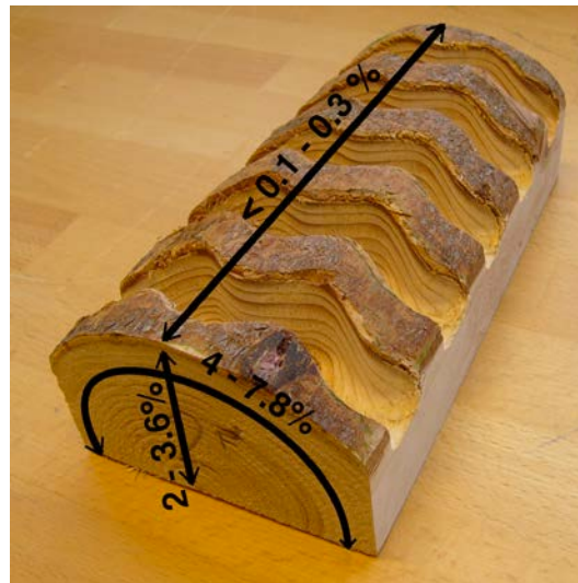
Figure 15. Orthotropic shrinkage in Norway spruce
