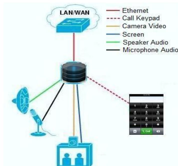
Figure 3. Illustrated telepresence system to be installed at an airport
