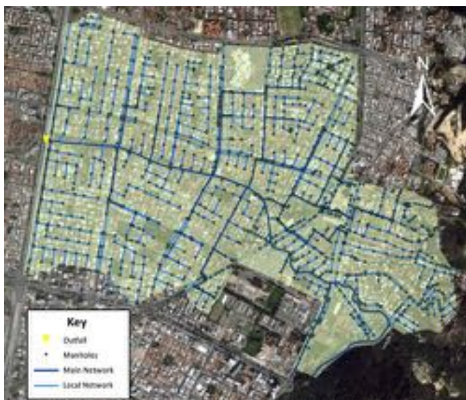
Figure 1. North Chicó sewerage network.
