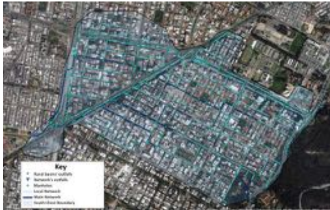
Figure 2. South Chicó sewerage network.
