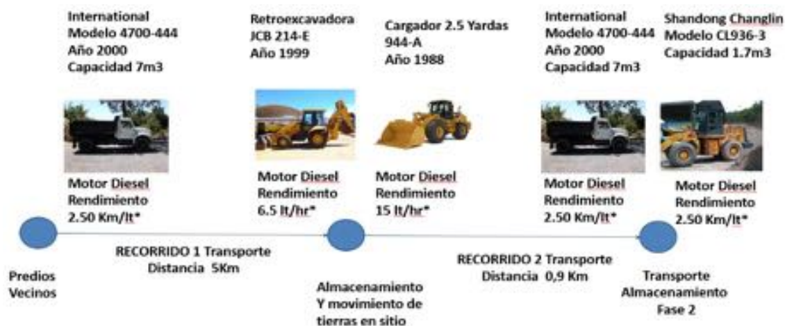
Figure 5: Analysis of the machinery used in the process "Extraction and maturation of open clay", according to its performance and characteristics. Source: self-made.
