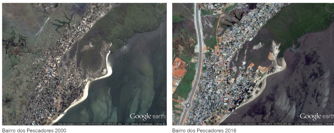
Figure 5. Ring road construction and progressive landfill and occupation of the Incomati floodplain at Bairro dos Pescadores (years 2000 and 2016 comparison)
