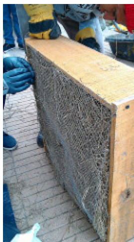
Figure 6. Second Panel, Hay between two steel mesh.
