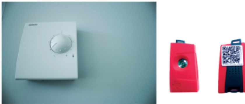
Figure 6. Thermostat for temperature regulation (left) and wearable smart sensor (right) for temperature and humidity measurements used in the ComfortSense Project
