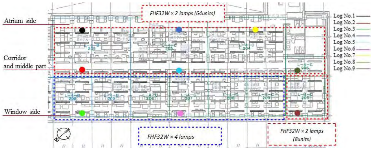
Fig3. Details of office layout, lighting circuit and place of lux loggers
