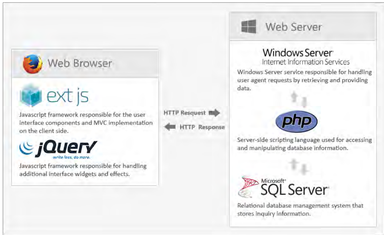
Figure 1 – SPS technological architecture
