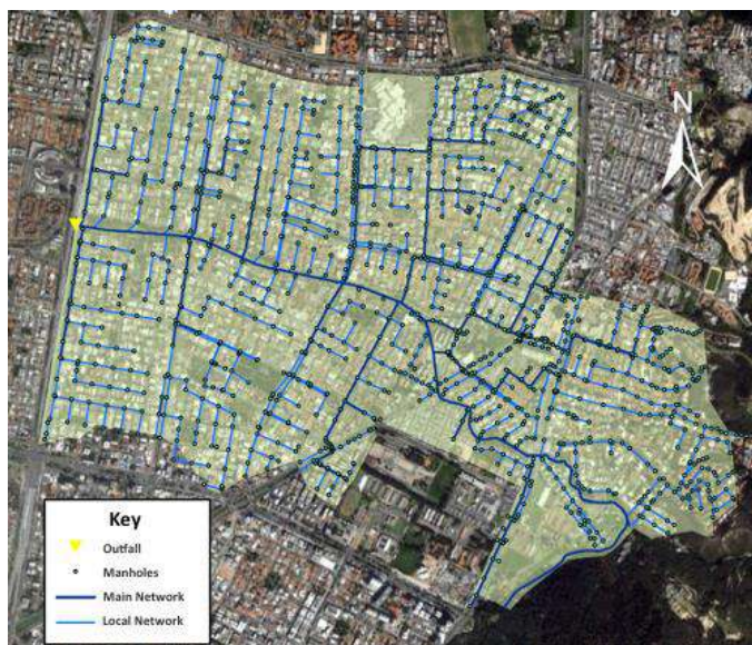
Figure 1. North Chicó sewerage network.
