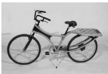
Figure 1. Wooden bike model developed by the GED research group.
