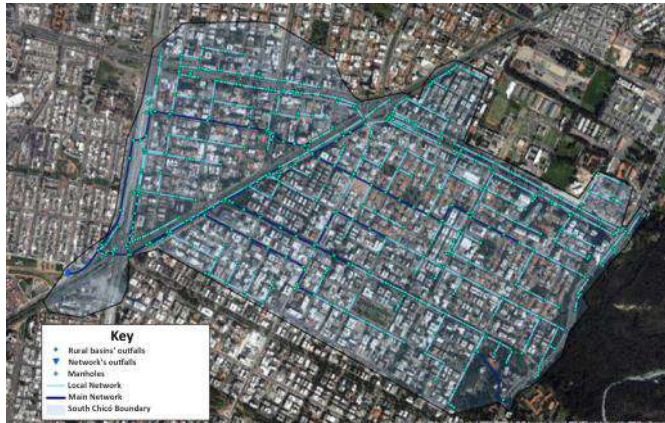
Figure 2. South Chicó sewerage network.
